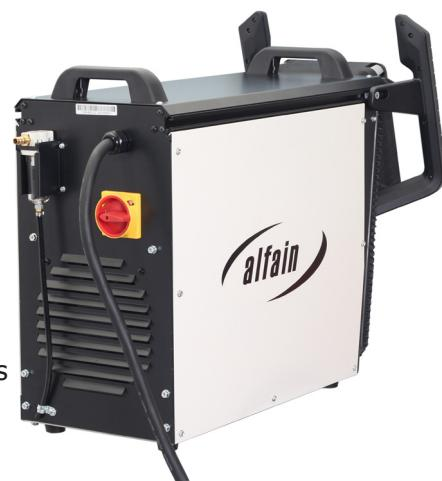
SVAROG 85 PLASMA is designed for high-quality cutting of materials up to 25 mm thick carbon steel. Productive cutting of carbon steel can be to the thickness of 20 mm. At lower demands on the quality of the cut can be cut through (separate) the material thickness to 35 mm.
