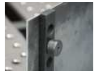
Magnet keeps sheet metal in vertical position
