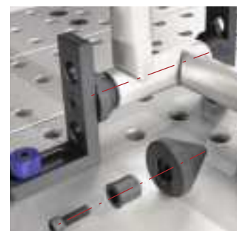
Horizontal application using Locking Pin
