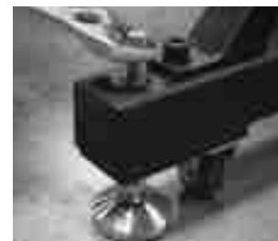
Large leveling pads with wrench flats
