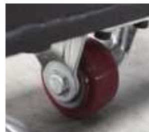
Two casters for quick repositioning of manipulator.
